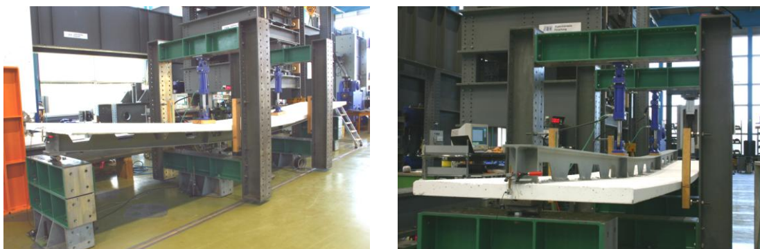
Figure 6 – Bending test with composite beam I (left) and beam II (right)
