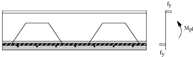
Figure 10 – Model for the calculation of the plastic resistance moment  $M_{pl}$  of the composite beam II with concrete slab on the bottom
