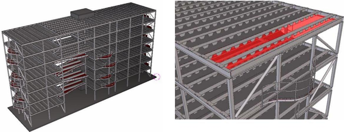
Figure 12 – Steel-structure of the planned residential building in Lugano, Switzerland using the novel type of composite slab system
