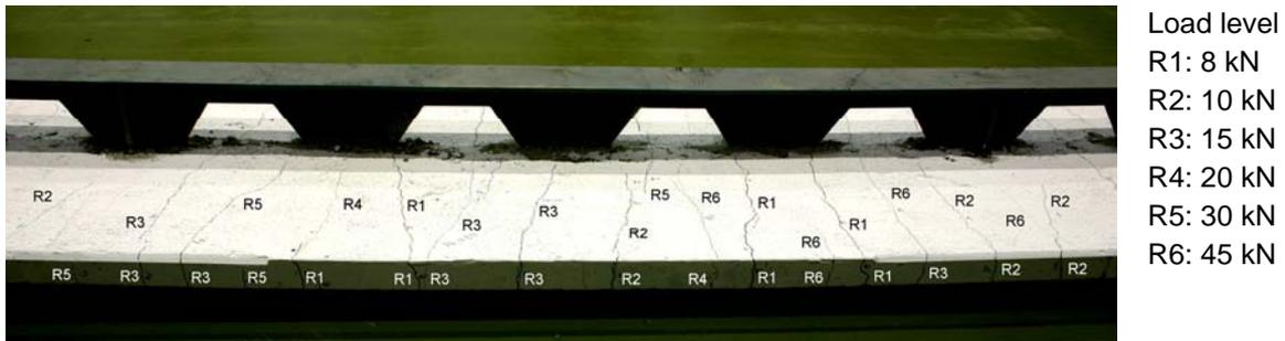
Figure 7 – Observed cracks on the concrete slab
