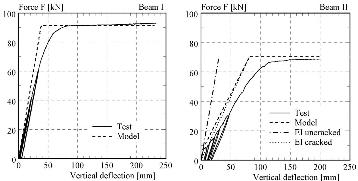
Figure 9 – Comparison between test results and simple calculation models
