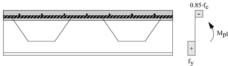
Figure 8 – Model for the calculation of the plastic resistance moment  $M_{pl}$  of the composite beam I with concrete slab on top
