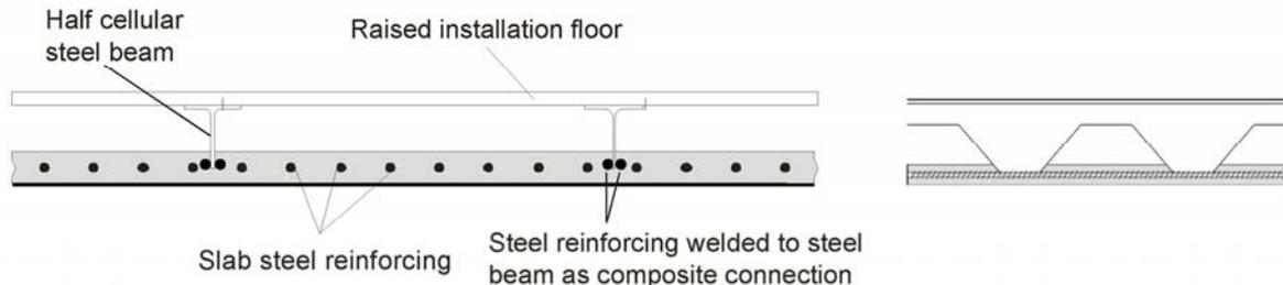
Figure 1 – Novel type of composite slab with integrated installation floor using cellular beams: the concrete slab is placed on the bottom
