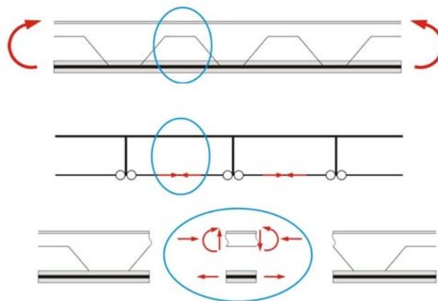
Figure 13 Calculation model for local bending of the steel section caused by shear forces
